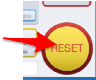
Figure 67: Reset to disable spindle relay
