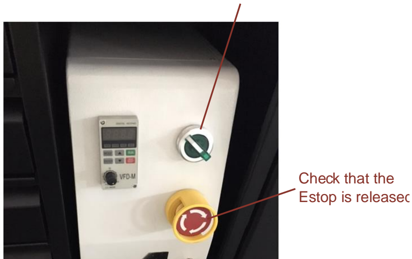
Figure 18: Green power switch and estop on the controller
